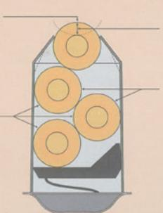
Three times the normal bolt-to-cartridge engagement ensures smoother, positive feeding.
